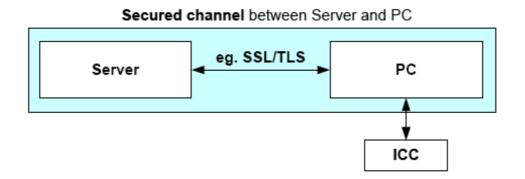
In the above example (taken from EN 419212-2), client/server authentication establishes a secured channel between a remote server and a PC. The ICC will be used as a cryptographic toolbox in order to provide the cryptographic functionality to the PC. If a process needs a certificate from the card that is not provided by OpenPGP (e. g. x.509), then it can be stored in the DO 'Cardholder certificate' (7F21 AUT) as 1st occurrence.
