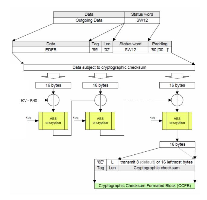
Response APDU computation of cryptographic checksum with AES in CMAC-Mode
