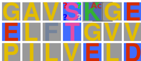
Figure 8.12: Rendering of a monomer modification in a polymer sequence. This figure shows how the chemical modification of monomer(s) is graphically rendered. The ‘K’ residue is modified using an “Acetylation” modification. The ‘S’ residue is modified with a modification that has no associated graphical vignette. The default vignette is thus used.
